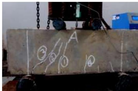
**Fig.6 Crack Pattern of CB**
