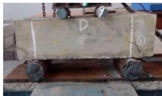
**Fig.7 Crack Pattern of RSXB**
